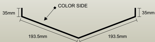
Fig.19. Illustration of sizes & types of roofing accessories.
